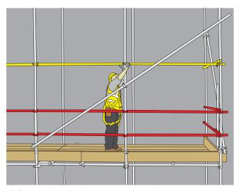
(i) Guardrail installed in advance to provide a safe zone for the dummy lift.
