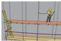
(ii) To traverse, double lanyards are used to remain continually attached, ideally to the inner standards or ledgers.
