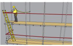
(iii) Progressively install guardrails (including stop-ends etc.) remaining continually attached to create the scaffolders' safe zone.
