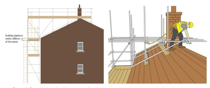
Figure 46: Example of a roof saddle sequence of work with eaves edge protection and continual attachment and eaves edge protection.
