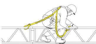
Figure 8: These illustrations show examples of the inherent risk of a fall in scaffolding where personal fall protection equipment will be the primary method of fall protection (e.g. (i) raising and lowering boards and (ii) working without a scaffolders' safe zone).
