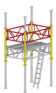
Figure 55: Fully decked and guardrailed working platform to form a **scaffolders' safe zone** with safe access and egress, used for the erection, alteration and dismantling of a formwork system.
