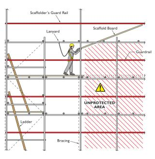
Figure 56: A Scaffolder raising platform boards to the next lift above working progressively backwards towards the ladder access.
