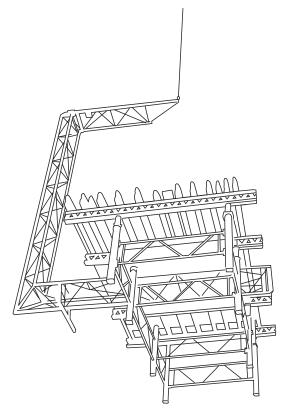
Figure 54: Formwork system erected on the ground or slab and lifted into position to avoid the need to work at height.
