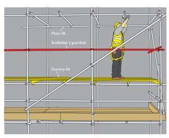
(ii) Dummy lift installed to enable fixing of the floor height lift.
