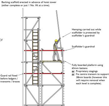
Figure 49: Debris chute or hoist tower construction.
