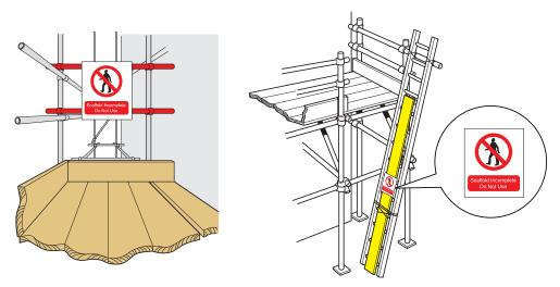
Figure 17: Restricted access. Shows examples of incomplete scaffolds with access restricted by physical means and warning signs restricting access to authorised scaffolders ONLY!
