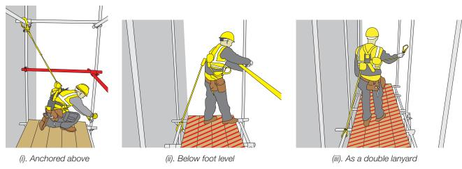
Figure 78: Examples of a hybrid self-retracting lanyard system in various scaffolding applications.
