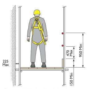
Figure 11: A finished working platform for users
