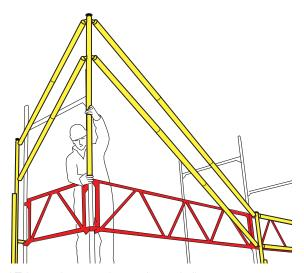
i Telescopic type advanced guardrail system
