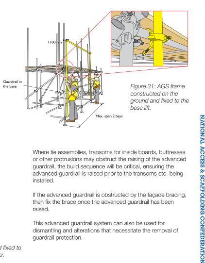
Where tie assemblies, transoms for inside boards, buttresses or other protrusions may obstruct the raising of the advanced guardrail, the build sequence will be critical, ensuring the advanced guardrail is raised prior to the transoms etc. being installed.
