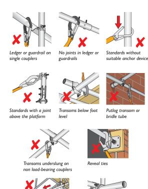
Figure 73: Examples of unsuitable anchor points.
