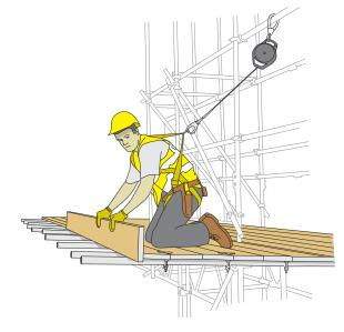
Figure 44: Falling object protection fan erected using an inertia reel.
