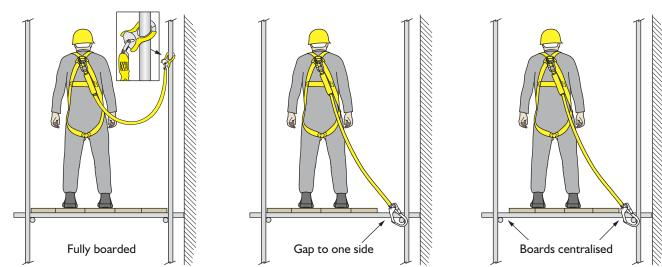
Figure 14: Fully boarded platform with a maximum of one board gap (225mm) may be permitted only if required to access the ledger below the platform as an anchor point.
