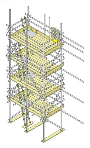
Figure 58: Ladder access bays with single-lift ladders.
