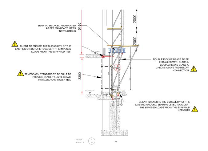
Figure 7: Extract from a drawing showing hazard warning.
