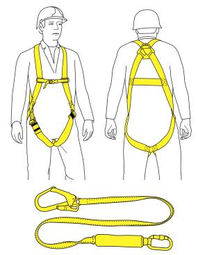
Figure 62: A minimum suggested personal fall arrest system.
