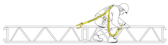
Figure 69: Scaffolder using a twin-tailed energy absorbing lanyard.
