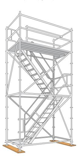
Figure 57: Typical proprietary system scaffold stairway.
