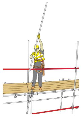
Figure 18: Illustration shows a scaffolder hemping a standard over a guardrail.
