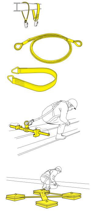
Figure 75: A selection of special connectors and anchor devices.
