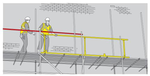
ii. Horizontal type advanced guardrail system
