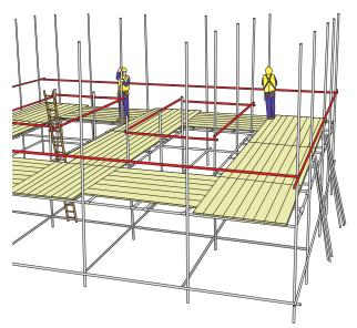
Figure 40: Example of a birdcage scaffolding system of work. Shows the **scaffolders' safe zone** used in runs for the erection of birdcage scaffolding. All bays can be reached to fix ledgers, transoms and braces without the requirement to fully board the entire structure.
