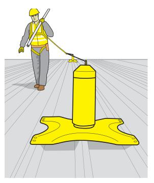
Figure 53: Scaffolder utilising an installed fall protection system for roof access.
