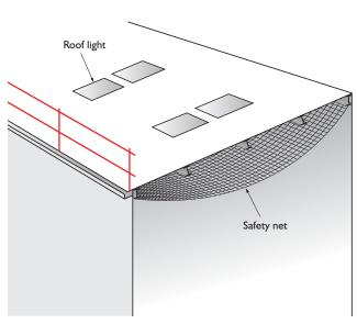
Figure 52: Fall arrest netting rigged to protect against falls through a fragile roof light.
