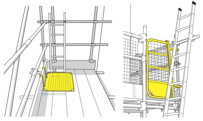
Figure 59: Internal ladder access with a protected ladder trap an example of good practice.
