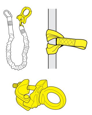
Figure 74: Anchor devices These pictures illustrate the use of connectors specifically developed for use as anchor devices to scaffold standards.
