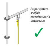
Figure 72: Examples of suitable anchor points.
