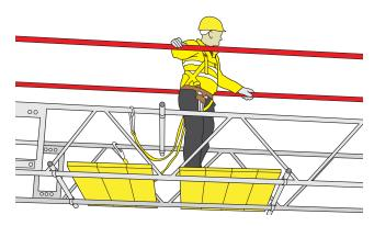
Figure 41: An example of bridging with beams using a double lanyard, temporary boarding and scaffolders' guardrails.
