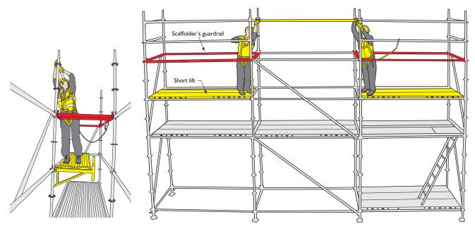
Figure 22: System scaffold side brackets used to create a scaffolders' step platform in alternate bays. The middle bays can be reached from adjacent bays to fix the guardrails.
