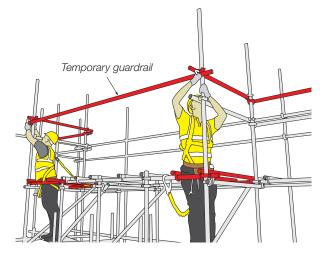
Figure 43: Temporary guardrail to maintain a **scaffolders' safe zone** for loading bay gate installation and removal. The temporary guardrail is removed once the gate is installed.
