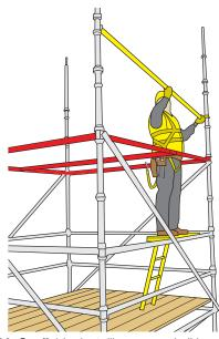
Figure 20: Scaffolder installing a guardrail in advance to the next lift from a scaffolders' step protected by the ledgers and transoms.
