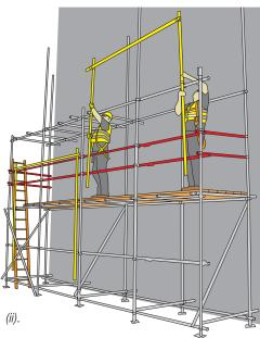
Figure 30: AGS frame constructed on the ground and fixed to the base lift. (i). Releasing the guardrail from the ledger. (ii). Raising the guardrail to the next level.
