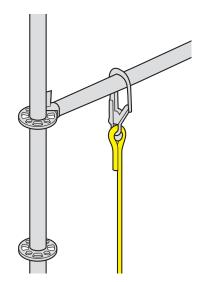
Figure 35: An example of an anchor point for a proprietary scaffolding system as per the manufacturers' instructions.
