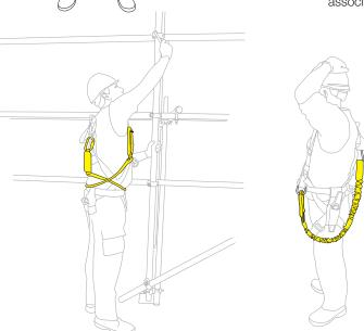
(i). A conventional fixed-length lanyard wrapped around the body and secured when not in use.
