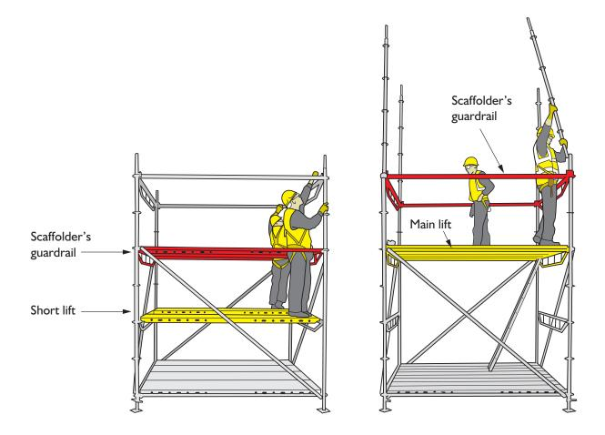
Figure 29: This sequence shows the short-lift system used to erect a system scaffold tower.
