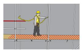
(v) The process is repeated, progressively installing guardrails to create the **scaffolders' safe zone** whilst remaining continually attached.
