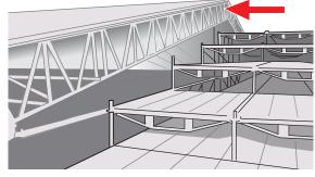
(ii.) Wide gable-end bay scaffolding bay is provided for erecting roof sections from a **scaffolders' safe zone**. Modular sections are rolled out on special rail and caster systems, to avoid the need for scaffolders to crab the beams.
