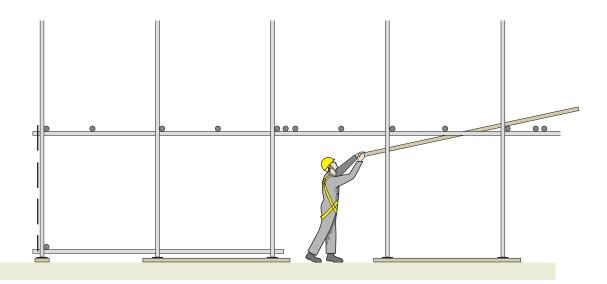
Figure 15: Boarding out first lift from below.
